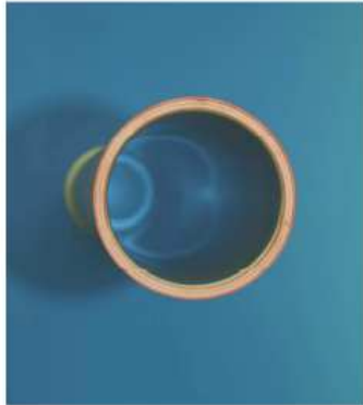
Tube piece for input and output section with cooper gasket
