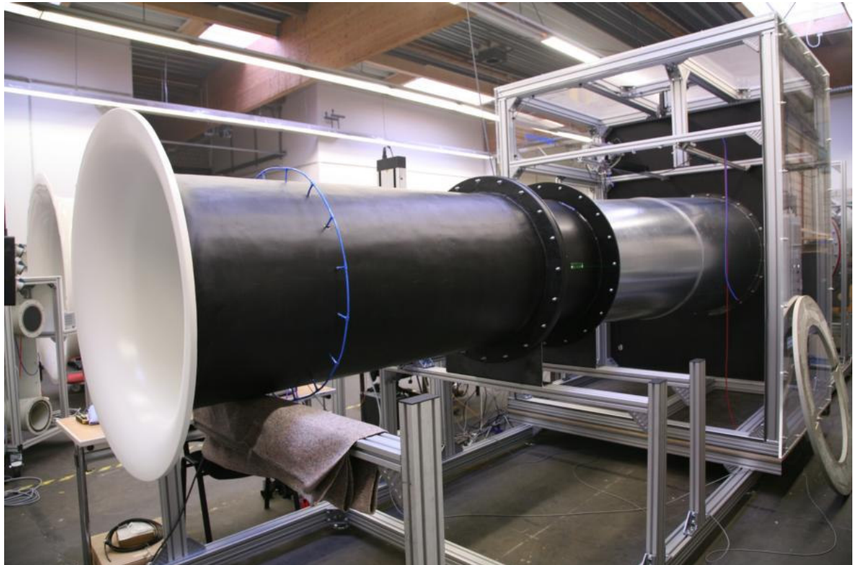
Fig. 1 Inletmeasuringnozzle made of GRP, diameter 700 mm
